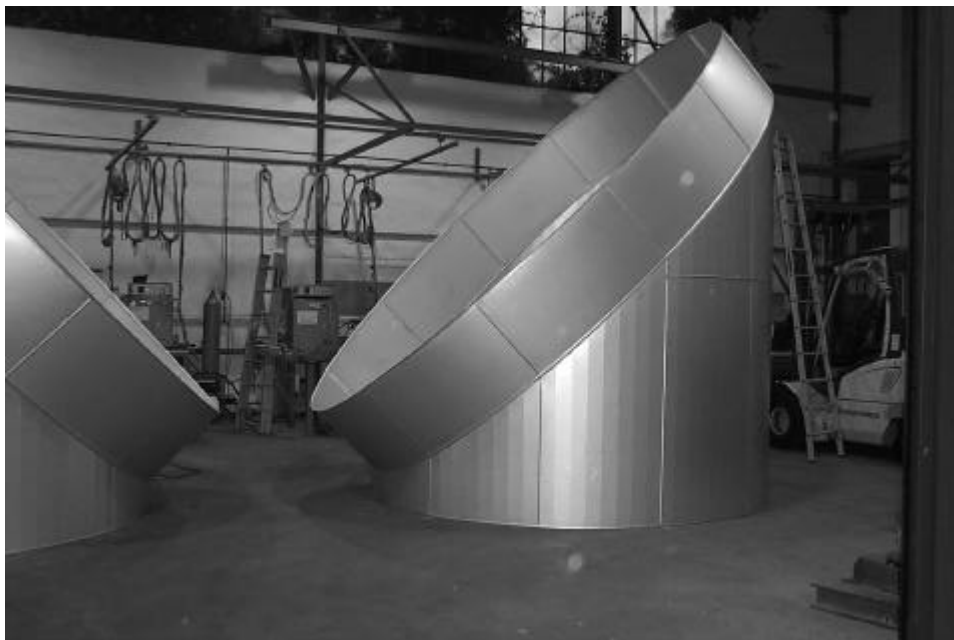
Figure 5: external steel cladding for a portion of the acoustical insulation system realized for the exhaust steam duct
